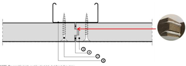
NOTE: The panel front side must be absolutely dust-free before gluing. .
