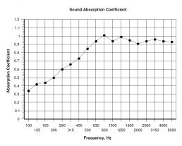
The absorption values illustrated illustrate the effectiveness of the system and serve acousticians and building physicists to determine the optimum reverberation time in the room. The measured values are based on laboratory measurements, which can vary depending on processing and object conditions.
